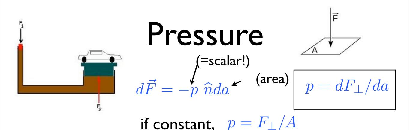
**Ex: hydraulic press**: pressure of fluid inside is almost constant (more soon), so  $p = F_1/A_1 = F_2/A_2$
