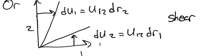
• So we have two  $3 \times 3$  tensors: the stress tensor  $\sigma_{ij}$  related to the forces, and the strain tensor  $u_{ij}$  related to the displacements. For a small displacements, Hooke's law linearly relates forces to displacement, as in the case of a spring. More generally, it linearly relates  $\sigma_{ij}$  and  $u_{ij}$ :
